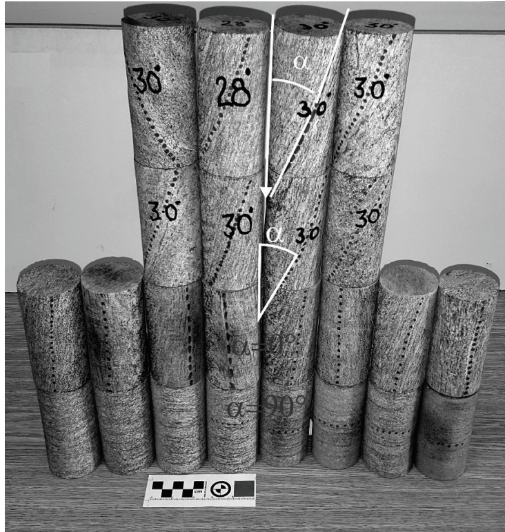
Figure 6. The relationship between loading direction and schistosity planes ( \alpha : anisotropy angle).
